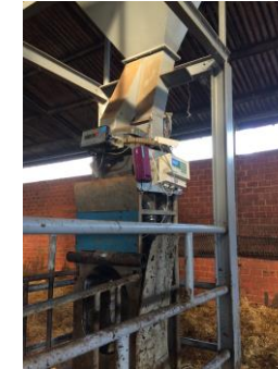
The device measuring the methane was set up on the ACS
