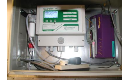
The device (Guardian®) allowing methane emissions measurements at the ACS
